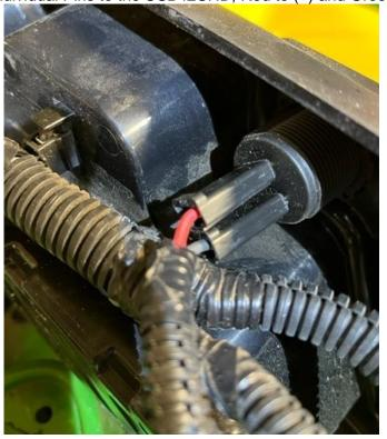
9. Before screwing the Panel into place, test to ensure the USB42CHD is able to charge a Phone and/or Device.
