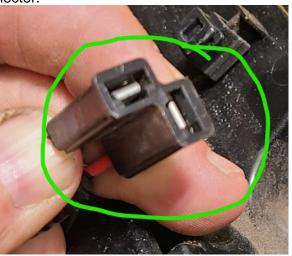
5. Next, remove the Plastic Housing from the Pins.
