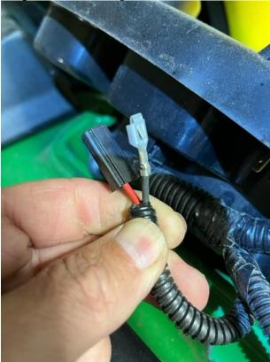
7. To remove the Receptacle, squeeze the tabs on either side and push through the Panel.
