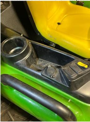
2. Screws and Bolts to remove the Panel to gain access to the 12V Receptacle will be in the underside of the Fender.
